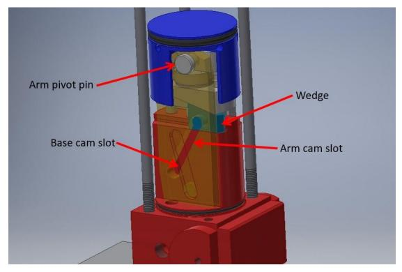
The cam arms do not allow the wedges to move backward after it's clamped, locking it in place.
